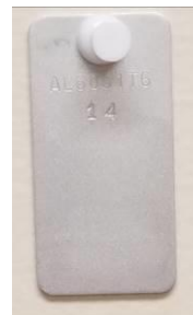
Figure 3: Aluminum corrosion test result for Naxonac®817LF
